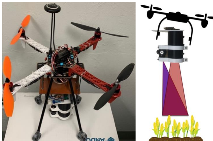
Figure 3.17 (left) Sensor unit integrated with the UAV using 3D printed and lab made parts. (right) Pictorial demonstration of data collection while in flight
